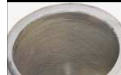
Cylinder Liner ID Surface Liner crosshatch surface clearly visible below the top ring turnaround is a good indicator that the engine maintained low wear, blow-by and good oil consumption control.
