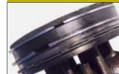
Typical upper piston ring belt Test engine shows very good piston deposit control with no crownland raking.
