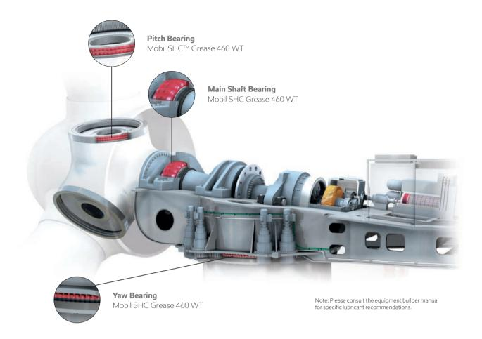
Versatile Mobil SHC™ Grease 460 WT synthetic grease enables you to use one product for main, pitch and yaw bearings, minimizing the risk of relubricating with the wrong product and allowing you to simplify your lubricant inventory.
