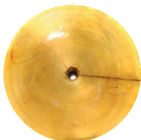
Mobil SHC Cibus™ 46: pass after 1,250 hours
