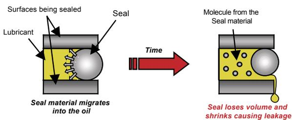
**Seal swell** – lubricant components migrate into the seal matrix. Moderate seal swell is welcomed whilst over swelling can cause deformation and leakage.
