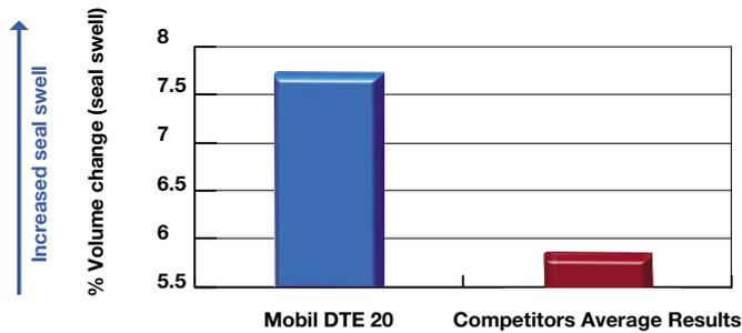
Mobil DTE 20 is designed to provide extra seal swell properties as demonstrated by the results of this test. This higher swell tendency, which is within manufacturers guidelines, can help reduce oil leakage resulting from oil/seal interactions.
