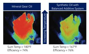
Tested using the Mobil  $^{\!\mathsf{TM}}$  Research modular small worm gear test stand.
