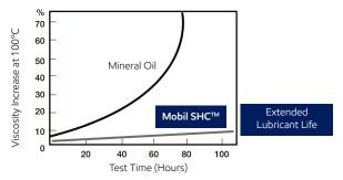
Comparison of Mobil  $SHC^{TM}$  versus a mineral oil in oxidation stability testing.
