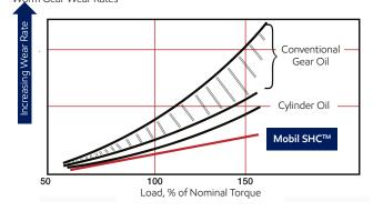
Tested using the Mobil™ Research worm gear test rig.
