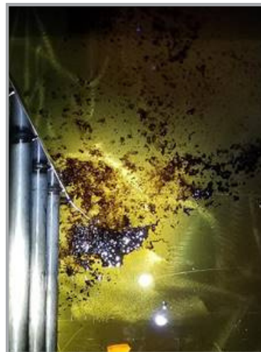
Figure 1. Contamination in Lube Oil Reservoir
