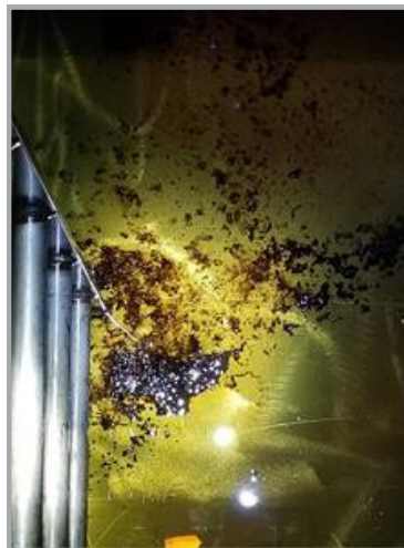
Figure 1. Contamination in Lube Oil Reservoir
